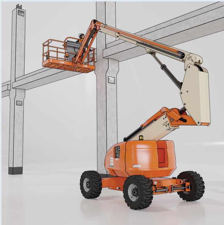
Figure 2 – Example of an EWP being used for a task at height
