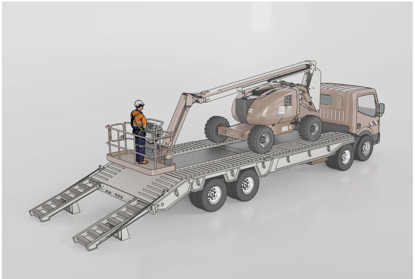
Figure 18 – Example of a delivery driver operating an EWP on a delivery vehicle
