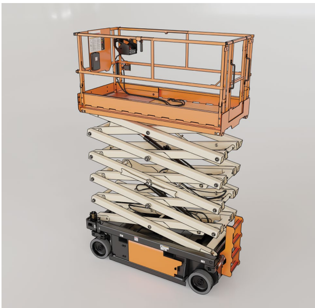
Figure 3 – Scissor-type EWP for operating on a flat or solid surface
