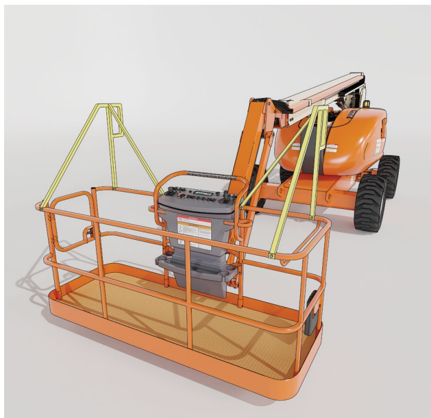
Figure 22 – Example of a physical barrier attached to the platform
