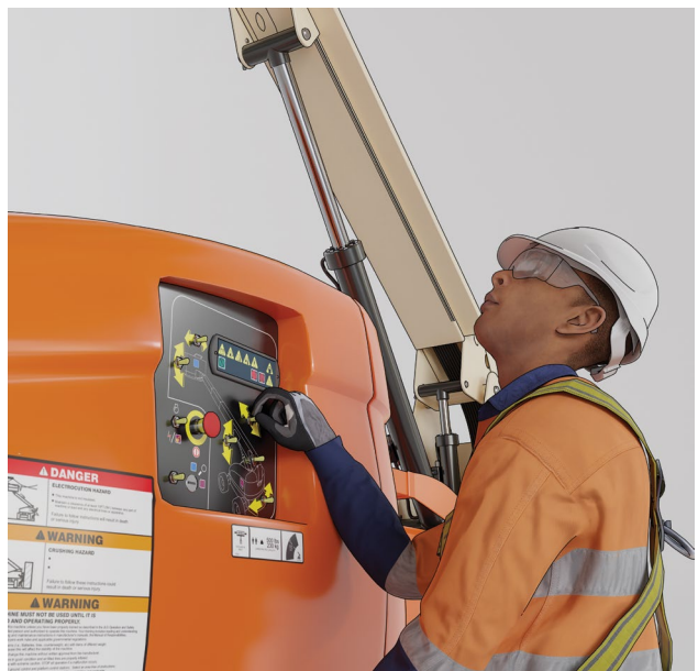
Figure 39 (b) – Example of emergency descent devices and ground based controls
