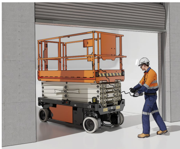
Figure 36 – Example of an EWP being walked through a doorway
