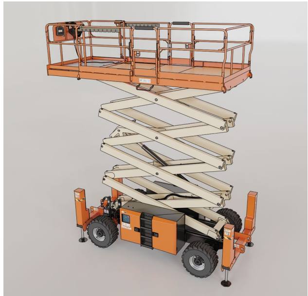
Figure 4 – Scissor-type EWP for operating on rough terrain or uneven surfaces
