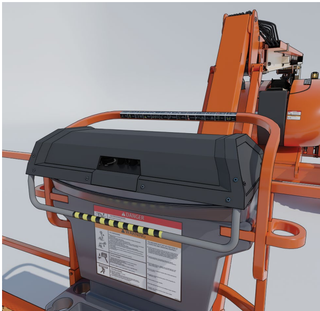
Figure 34 – Example of an EWP control protection
