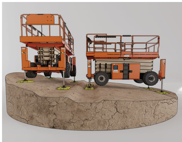
Figure 37 – Scissor-type EWP outriggers lowered into steps created in a slope
