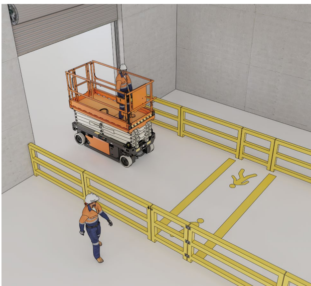
Figure 29 – Example of traffic management controls
