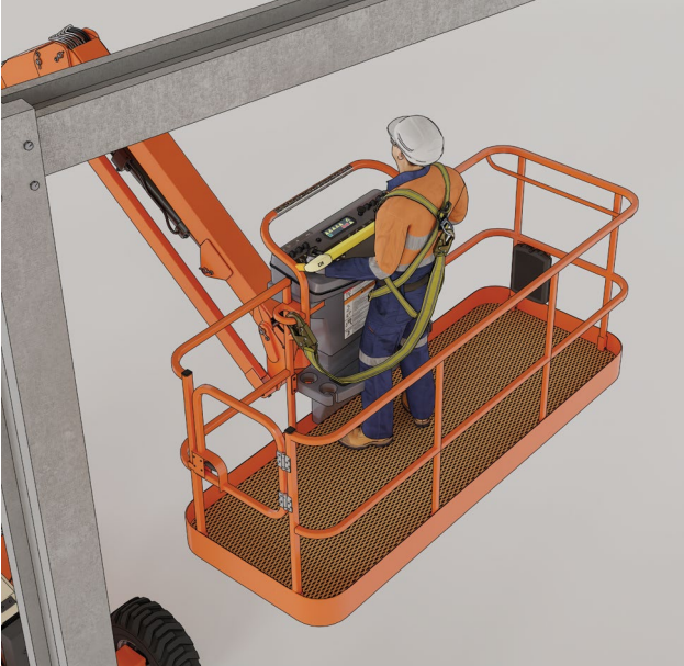
Figure 21 – Example of an EWP working near overhead structures fitted with a pressure sensing device
