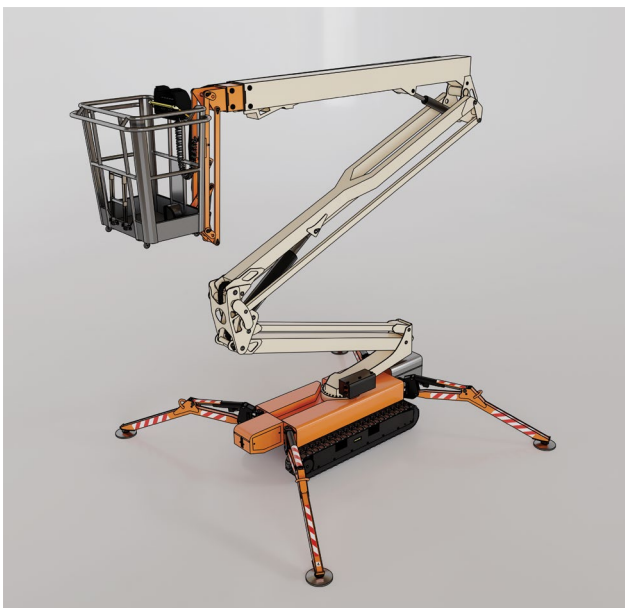
Figure 9 – Spider lifts or compact crawlers for sites with restricted access
