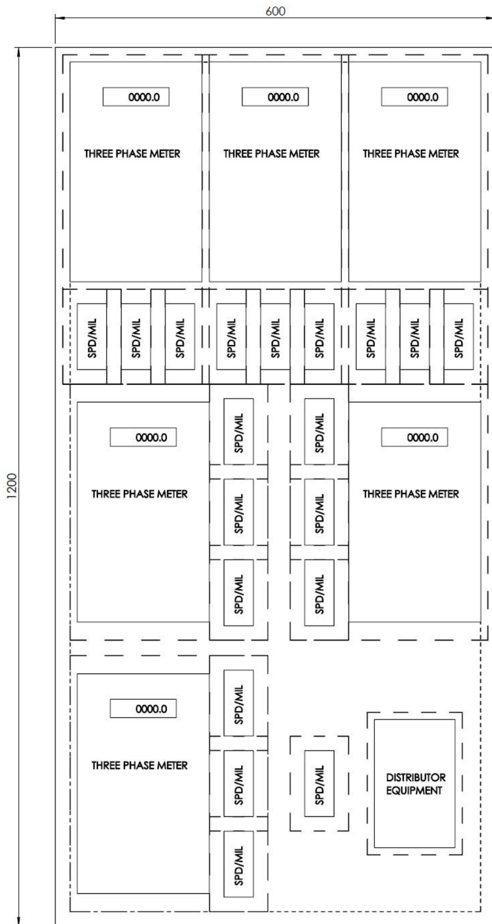
Figure 22 - Typical Panel Layout for Multi Occupancy, multiphase, 1200 x 600 panel
